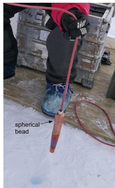
Figure 2. Heated copper “plumb bob” for melting and glazing the first 6 m of the firn hole.
