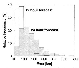
FIG. 6. Forecast error (rms error; km) distribution for 12- (thick line) and 24-h (thin line, shaded) forecasts provided by the analog ensemble prediction model (optimal metric with N = 20 ensemble members).
