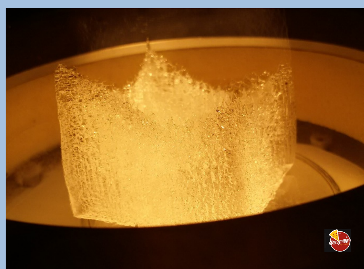
Photograph of ice after sublimation. The preliminary set-up with an IR-bulb reached a sublimation rate of 2 cm/hour. In order to maintain a more homogenous sublimation front an NIR-Laser with beam shaping optics will replace the bulb.
