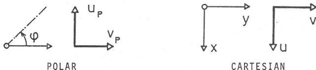
Figure 6.4 Coordinate systems and position of the components of the velocity field. The systems are located in the centre of curvature.
