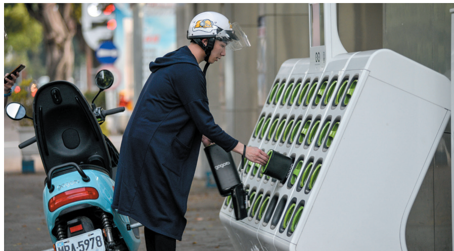
A rider swaps scooter batteries at a roadside facility in Taiwan.
